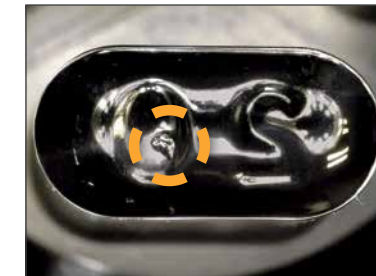
Punch Tip Damage Photo Taken with IN 7951
