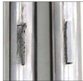
Damage to key from excessive wear
