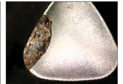
Punch Tip Damage Photo Taken with IN 7951
